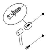
Insert the wall plugs into the holes before fixing the bracket to the wall using the supplied screws.
